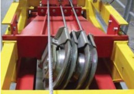
Verreet's wire rope testing machine in operation
